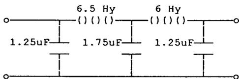
The inductors are large enough to block low-frequency, high-voltage telephone ringing current. Using the same inductors, the filter could be redesigned as an elliptic-function type, yielding 70 dB stop-band rejection with a deeper notch at 60 or 50 Hz.
