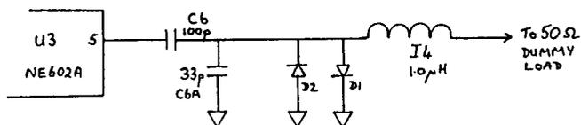
Testing the transverter after this modification indicated that a signal injected into the transverter was only 1/8 of the voltage for the same S-meter reading on the CB radio; a gain of 18 dB! Tests in the cave were even more impressive with the range being nearly doubled. We were able to use 2-way speech (SSB) to 280 m using the 1m antennas, and to 170 m using the 28 x 43 cm (11 x 17") antenna wound into the lid of the carrying case.
