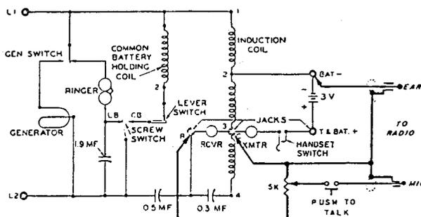
Telephone EE-8—schematic diagram.
