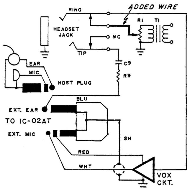
Fig. 2. Alternate wiring method: switch contacts in the closed-circuit headset jack connect the telephone interface to the VOX circuit whenever the headset is unplugged. T1 and R1 are mounted inside the VOX unit.
